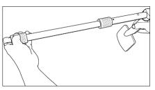
Loosen lower camlock and extend stem to desired operating length. Hand-tighten the camlock.
