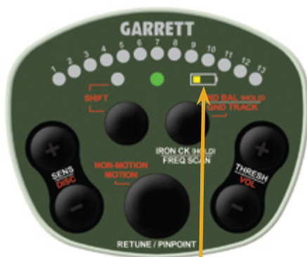
Low Battery Indicator
