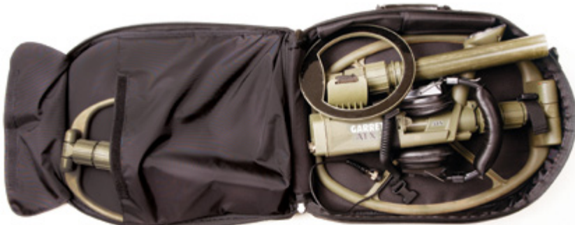
Figure 6: ATX with Deepseeker coil attached + DD coil + 8" mono coil + headphones. Note: close velcro flap to secure DD coil.
