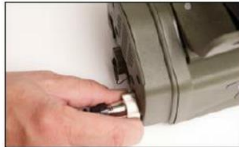
Hand-tighten connector collar.
