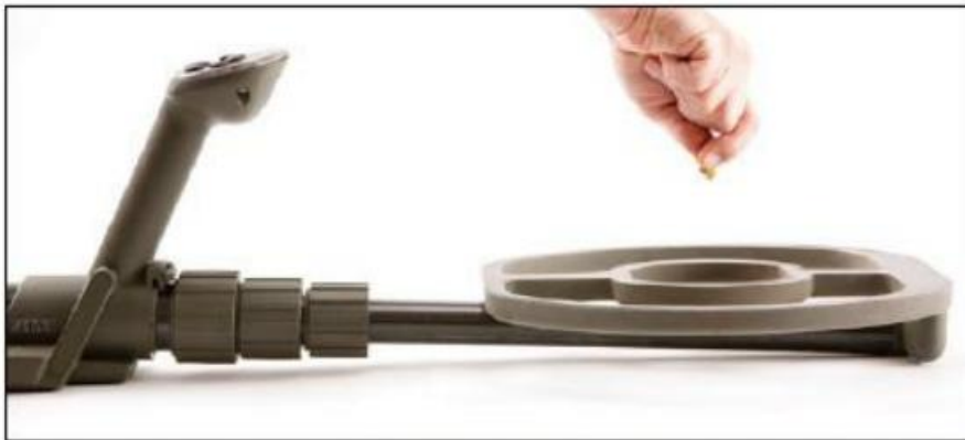
For bench testing, take the ATX outdoors, away from electrical interference and large metallic objects. Extend the first stem and lay the coil back as shown above.
