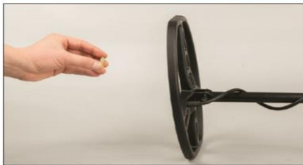
For bench testing, place the searchcoil on a flat, stable, non-metallic surface that is at least a meter from other metallic objects.
