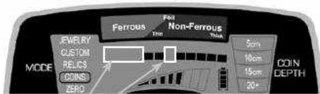
In COINS Mode, 4 pixels under ferrous and one pixel of foil are notched out.
