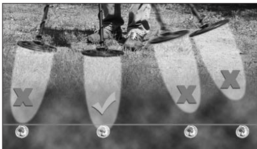
Figure 1D. This person is lifting his searchcoil off the ground at the end of his swing. As the coil moves away from the ground, it does not penetrate as deeply into the earth. In this illustration, three of the four coins would not be detected.
